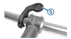
8 Press down slightly and turn the Edge device clockwise until it locks into place.
